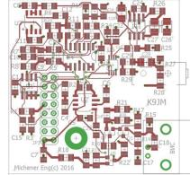
A direct conversion receiver that can be used to measure and sniff out RF noise sources. Audio monitor, digitizes audio, measures level in dB. Fixed bandwidth spectrum analyzer sweep with about 4KHz bandwidth.
